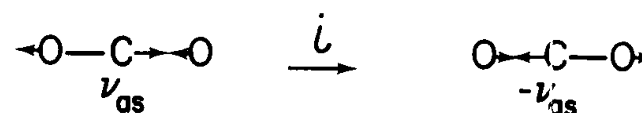
Fig. 3-34. The vibration \nu_{as} goes to minus itself upon inversion. That is, the direction of motion of each atom changes sign.
